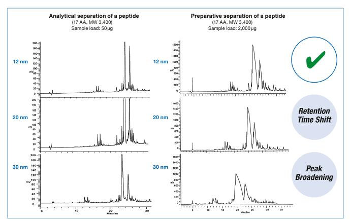
Therefore, the screening of different pore sizes with increased sample loadings is key to identifying the most appropriate pore sizes for an efficient purification process.
