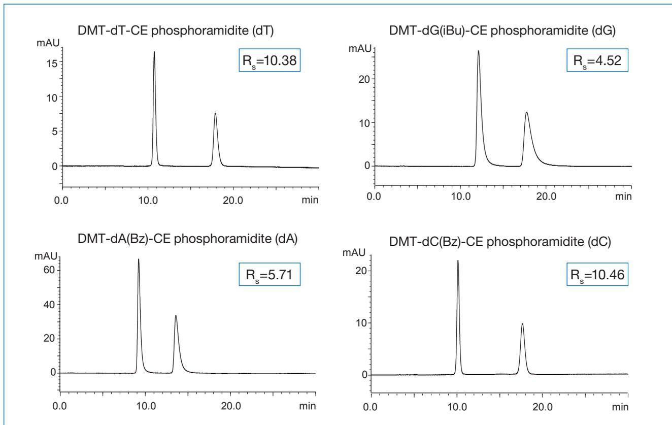
Figure 3: Separation of four phosphoramidites using NP conditions.
