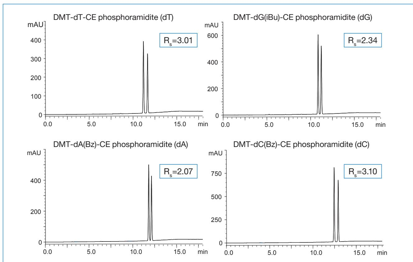
Figure 2: Separation of four phosphoramidites using RP conditions.
