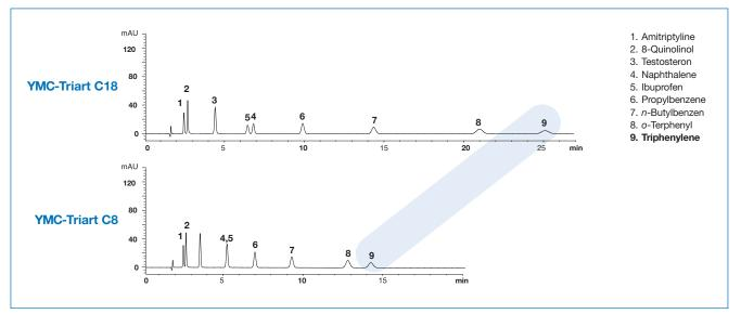
Figure 1: Comparison of the retention times using YMC-Triart C18 and C8 columns.
