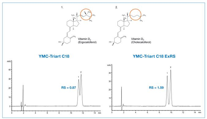
Figure 3: Separation of vitamin D<sub>2</sub> and D<sub>3</sub> using YMC-Triart C18 and YMC-Triart C18 ExRS columns.
