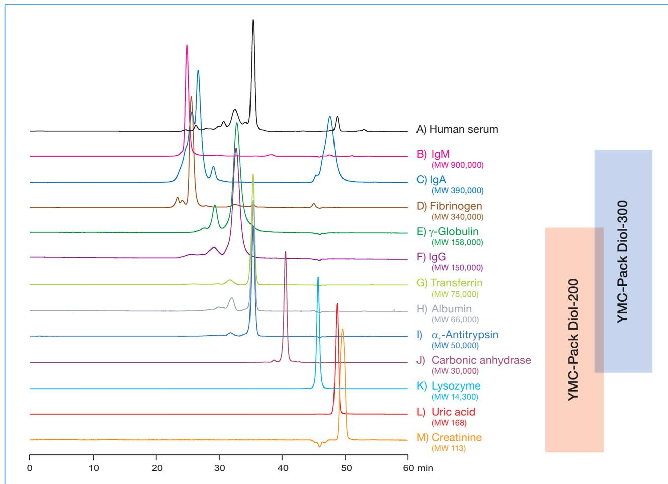
Figure 2: Analysis of plasma constituents by coupling two columns: **YMC-Pack Diol-300** and **YMC-Pack Diol-200**.
