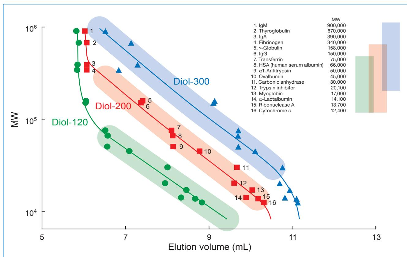
Figure 1: Calibration curves of YMC-Pack Diol-120, YMC-Pack Diol-200 and YMC-Pack Diol-300 for analytes with a molecular weight ranging between 12,400 and 900,000 Da.
