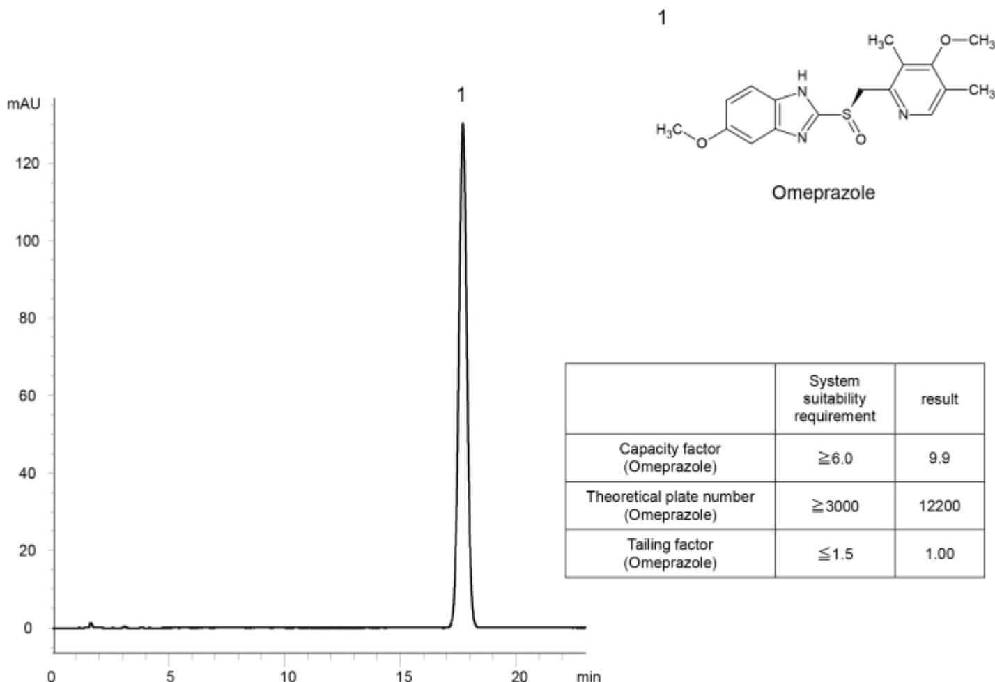
Column : YMC-Triart C8 (5 µm, 12 nm)
