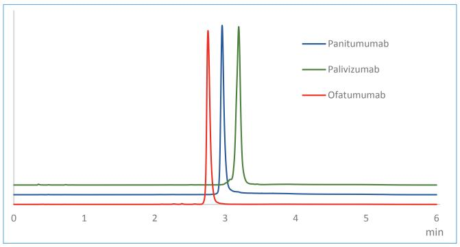
Figure 1: UHPLC analysis of different monoclonal antibodies using YMC-Triart Bio C4.
