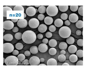
SEM pictures of the material before the first packing and after the 20<sup>th</sup> packing prove the high mechanical stability of the YMC-Trairt Prep materials.
