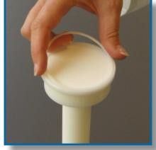
When replacing a frit, both a new frit and a new o-ring are required.
