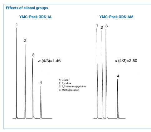
The separation factor (**a**) of internal standards methylparaben / 2,6-dimethylpyridine for YMC-Pack ODS-AL, which is not endcapped is different to that of YMC-Pack ODS-AM. Due to the residual silanol groups, YMC-Pack ODS-AL shows higher retention of pyridines.
