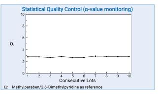
interactions with residual silanol groups. 2,6-dimethylpyridine, however, represents a lipophilic amine compound which has a high potential of unspecific interaction with unreacted acidic silanols. An increase in retention of 2,6-dimethylpyridine and hence lower  $\alpha$ -values would indicate incomplete C18 bonding and/or ineffective endcapping. YMC specifies for ODS-AM that the statistical  $\alpha$ -value of methylparaben and 2,6-dimethylpyridine be 2.77 +/- 0.20.
