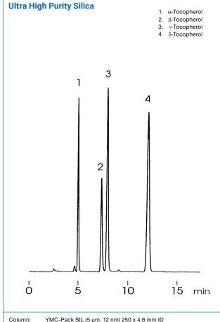
Column: YMC-Pack SIL (5 µm, 12 nm) 250 x 4.6 mm ID Part No : SI 12S05-2546WT
