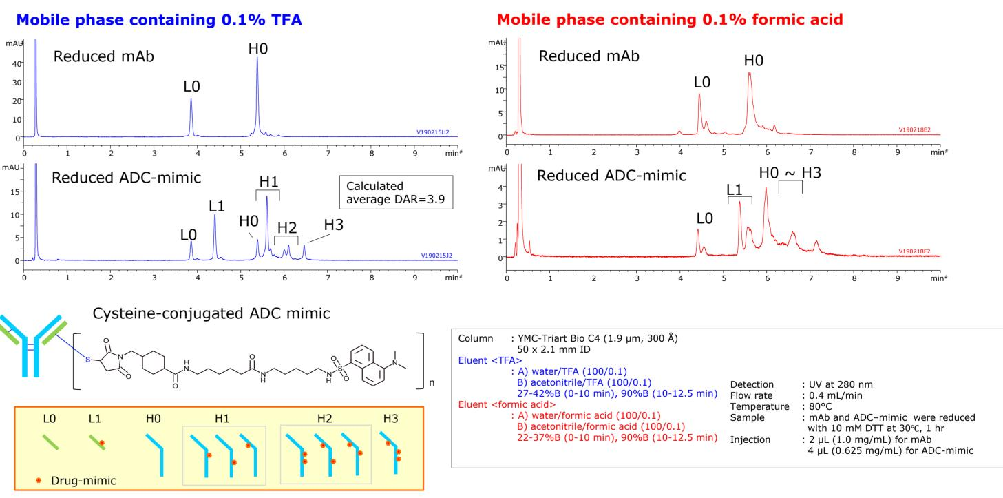
The analysis results of (A) mAb fragments, (B) intact mAbs, and (C) reduced mAbs and ADCs are compared between 0.1% TFA added condition and 0.1% formic acid added condition. The excellent resolution and peak shape are obtained with YMC-Triart Bio C4 and 0.1% TFA added condition for a variety of mAb and related substances which are different in their molecular size and hydrophobicity.
