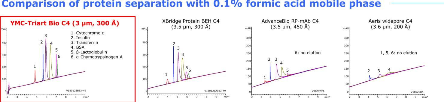
: A) water/formic acid (100/0.1) Eluent B) acetonitrile/formic acid (100/0.1) 10-95%B (0-15 min) : 40°C Temperature : UV at 220 nm Detection
