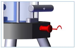
14. Loosen the locking bolts and lock them by turning slightly.
