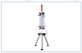
6. Lift the column body vertical from the column stand using two holding bars which are vertically above each other.
