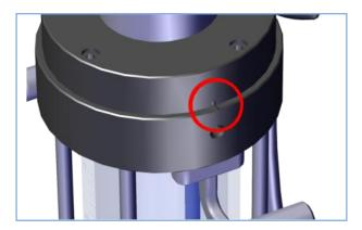
21. Align the marks on the closing disc (AEP) and column disc.
