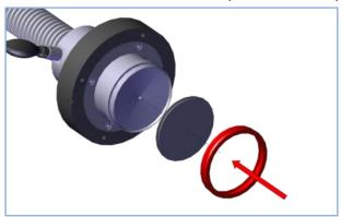
5. Reattach the profile gasket and press firmly in position.
