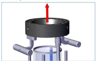
4. Remove column disc from the column body.
