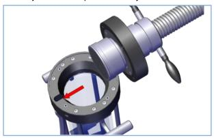
19. Put the piston of the adjustable end piece in a smooth angle opposite the drain function on the column body.
