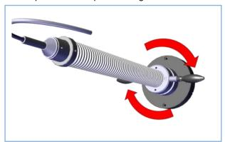
14. Turn the closing disc of the adjustable end piece in the UP direction as far as it will go.
