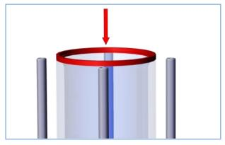
9. Put the flat gasket corresponding to the structure on the top edge of the glass body.
