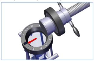
16. Put the piston of the adjustable end piece in a smooth angle opposite the drain function on the column body.
