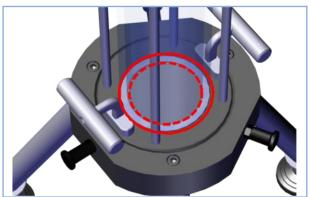
8. Check that the glass body is concentric with the gaskets.
