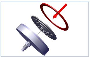
8. Reattach the ring gasket A and press firmly in position.
