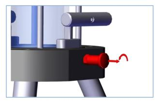
8. Loosen the locking bolts and lock them by turning slightly.
