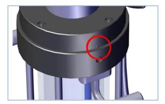
18. Align the marks on the closing disc (AEP) and column disc.
