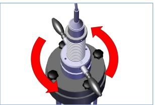
1. Turn the piston of the adjustable end piece in the UP direction as far as it will go.
