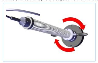
17. Turn the closing disc of the adjustable end piece in the UP direction as far as it will go.
