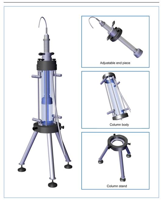
The YMC Pilot<sup>PLUS</sup> column consists of the adjustable end piece, the column body and the column stand. These parts can be assembled whilst operating the column without any tools.
