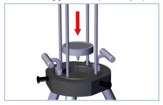
9. Replace the fixed end piece into the closing disc (CB).
