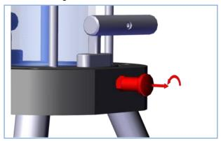
5. Loosen the locking bolts and lock them by turning slightly.
