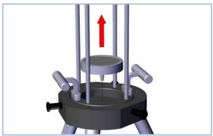
4. Press the fixed end piece with the connector out of the closing disc (CB).
