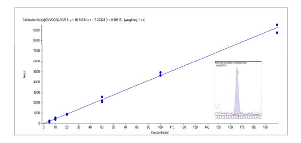
The calibration line obtained from the spiking of gliadin, a specific wheat protein, into gluten-free wheat from the range of 5–200 ppm for wheat peptide 3. Inlayed in the calibration line is the chromatogram for the 10 ppm spike of gliadin into gluten-free flour.
