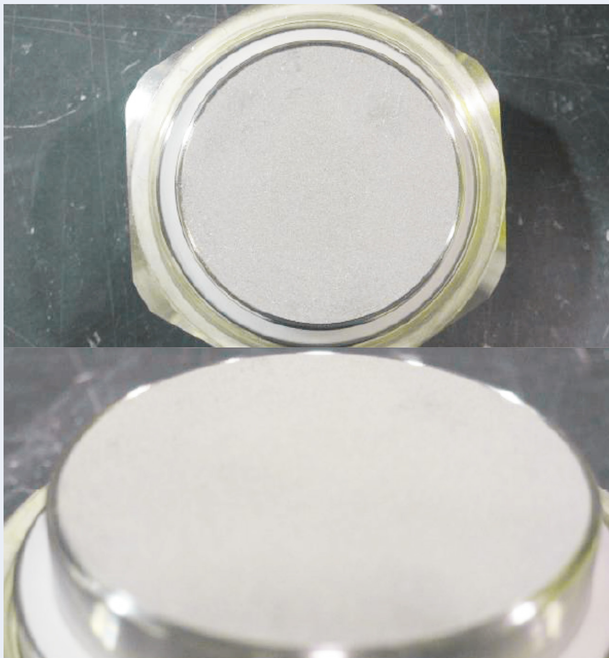
Figure 5: Open column with inlet frit after 1,000 injections
