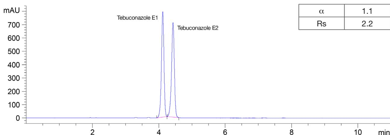
Figure 4: Separation of Tebuconazol enantiomers on **CHIRAL ART Cellulose-SC** (KSC99S03-1503WT, 3  $\mu\text{m}$  particle size, 150 mm  $\times$  3 mm), 0.43 mL/min, 25°C, 2  $\mu\text{L}$  (1 mg/mL) injection volume, water/ acetonitrile (40/60), 220 nm.
