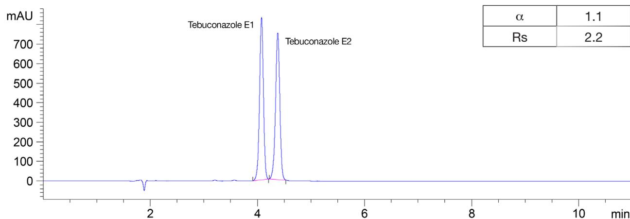
Figure 5: Separation of Tebuconazol enantiomers on **CHIRAL ART Cellulose-SC** (KSC99S03-1503WT, 3  $\mu\text{m}$  particle size, 150 mm  $\times$  3 mm), 0.43 mL/min, 25°C, 2  $\mu\text{L}$  (1 mg/mL) injection volume, water with 0.1% formic acid / acetonitrile (40/60), 220 nm.
