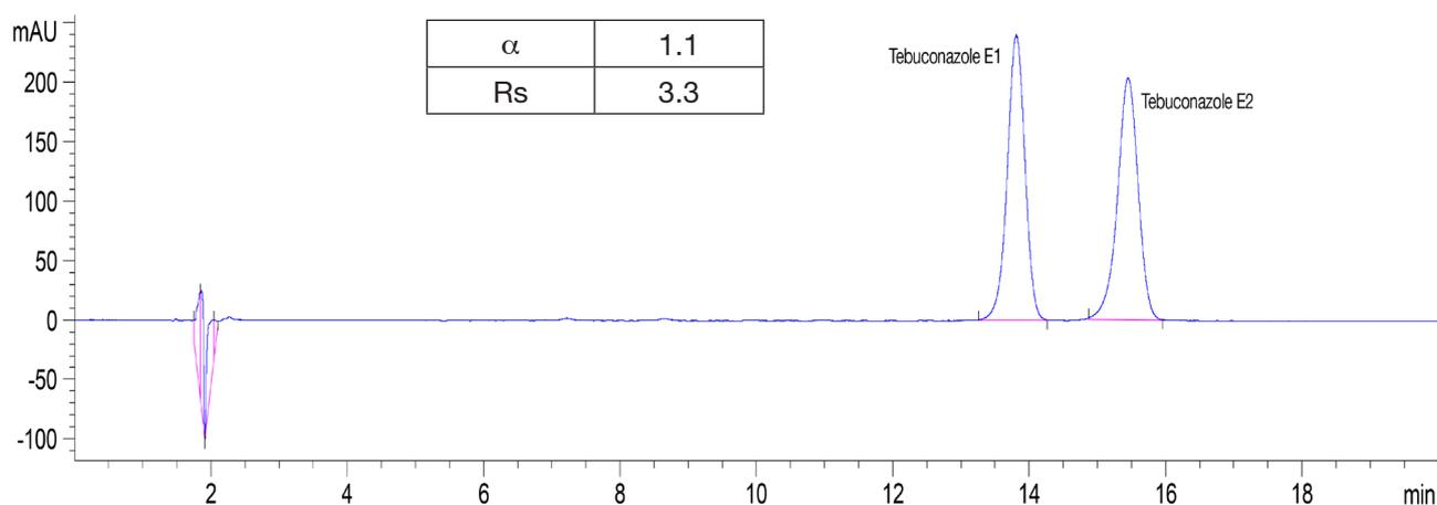
Figure 6: Separation of enantiomers Tebuconazole on **CHIRAL ART Cellulose-SC** (KSC99S03-1503WT, 3  $\mu$ m particle size, 150 mm  $\times$  3 mm), 0.43 mL/min, 25°C, 2  $\mu$ L (1 mg/mL) injection volume, water with 0.1% formic acid/ acetonitrile (60/40), 220 nm.
