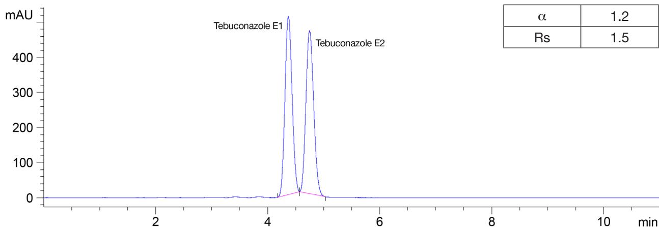
Figure 3: Separation of Tebuconazol enantiomers on **CHIRAL ART Cellulose-SC** (KSC99S05-1546WT, 5  $\mu$ m particle size, 150 mm  $\times$  4.6 mm), 1 mL/min, 25°C, 5  $\mu$ L (1 mg/mL) injection volume, water/acetonitrile (40/60), 220 nm.
