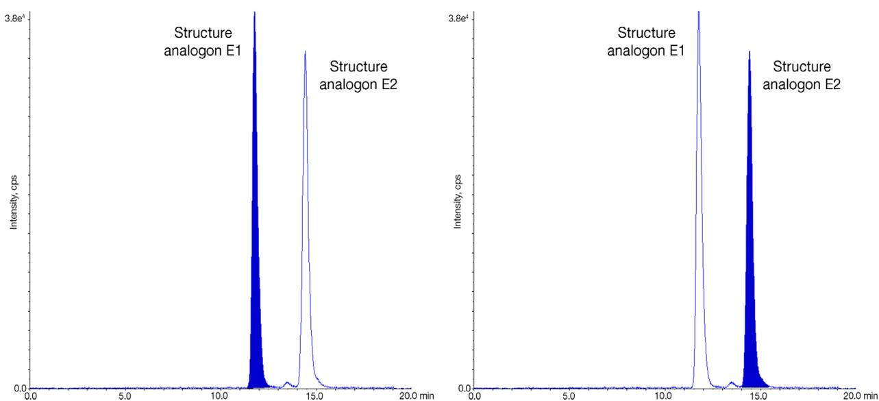
Figure 8: Separation of structure analogon enantiomers on **CHIRAL ART Cellulose-SC** (KSC99S03-1503WT, 3  $\mu$ m particle size, 150 mm  $\times$  3 mm), 0.43 mL/min, 25°C, 1  $\mu$ L injection volume, water with 0.1% formic acid/ acetonitrile (60/40); ESI+ m/z 312-70.
