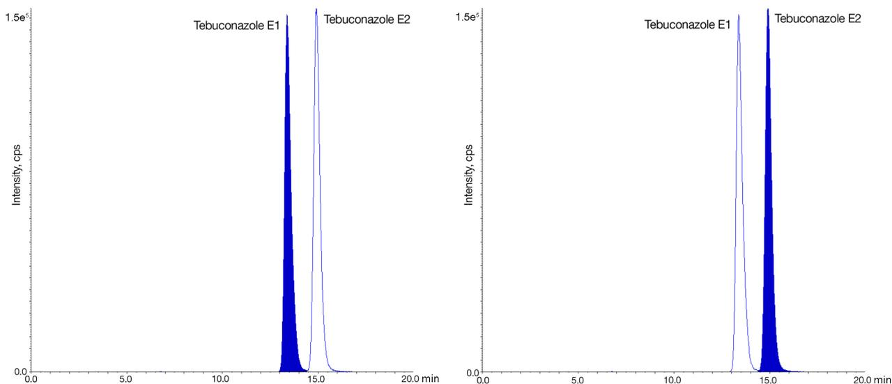
Figure 7: 250 µg/L Standard Solution; Separation of Tebuconazole enantiomers on **CHIRAL ART Cellulose-SC** (KSC99S03-1503WT, 3 µm particle size, 150 mm × 3 mm), 0.43 mL/min, 25°C, 1 µL injection volume, water with 0.1% formic acid/acetonitrile (60/40), ESI+ m/z 308-70.
