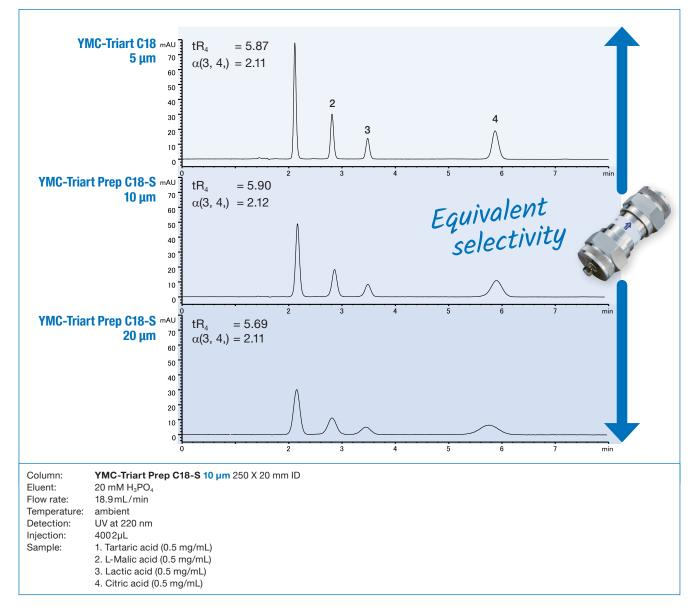
With YMC-Triart Prep, a pH stable preparative grade HPLC stationary phase is available. This hybrid material can be produced in lot sizes of up to several hundred kg. The robustness of the phase and its availability in multi-ton quantities makes it well suited for production scale applications. YMC-Triart Prep is chemically stable up to pH 10.0 which provides more flexibility for method development and also
