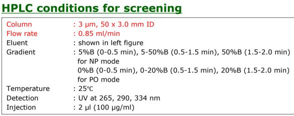
The suggested initial screening protocol and conditions in chiral HPLC are shown on the left. The combination of short columns packed with four types of 3 µm immobilised CSP and rapid gradient elution with 8 types of normal phase (NP) or polar organic (PO) mobile phases can be employed for chiral phase method screening for pharmaceutical compounds.
