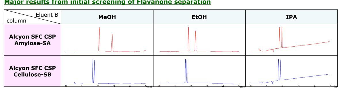
The acceptable resolution of Flavanone enantiomers was achieved within a short run time using Alcyon SFC CSP columns under all of the SFC screening conditions shown in the above chromatograms. The combination of Alcyon SFC CSP Amylose-SA phase and mobile phases consisting of  $CO_2/MeOH$  or  $CO_2/EtOH$  proved to give superior resolution.
