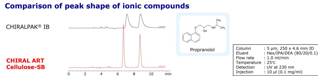
CHIRAL ART columns provide good peak shapes of ionic and metal coordination compounds.
