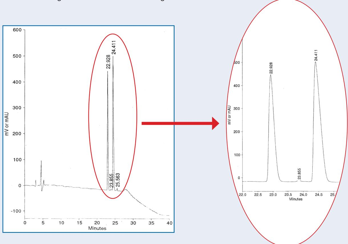
Separation of Angiotensin II and its modified form on YMC-Triart C8, 5 µm particle size, 12 nm pore size, 250 × 4.6 mm ID; YMC Part number: TO12S05-2546WT
