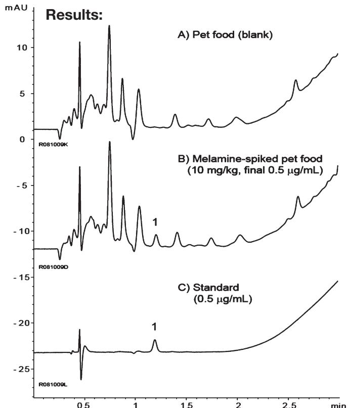
Säule: YMC-UltraHT Hydrosphere C18 (2 µm, 12 nm) 50 x 2.0 mm ID
