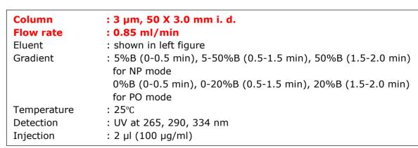
the rapid gradient elution of eight types of Normal Phase (NP) and Polar Organic (PO) mobile phase are employed for separation method screening of pharmaceutical compounds
