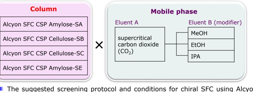
The suggested screening protocol and conditions for chiral SFC using Alcyon SFC CSP immobilized type columns are shown in above. They sometimes offer advantages over HPLC in a resolution and reduction of method development. The low viscosity of supercritical carbon dioxide can allow use of longer column with higher efficiency at higher flow rate, and also it enables great reduction of organic solvent consumption.
