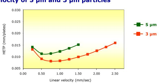
CHIRAL ART Cellulose-SB, 250 X 4.6 mm i. d. Hex/IPA(90/10) : 0.25, 0.50, 0.75, 1.0, 1.25, 1.50 ml/min for 5 µm 0.25, 0.50, 0.75, 1.0, 1.25, 1.50, 1.75, 2.00, 2.25, 2.50 ml/min for 3 um Detection : UV at 230 nm : trans-Stilbene oxide
