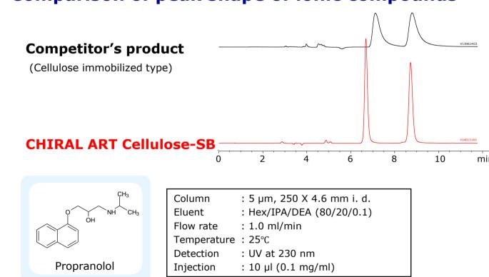
CHIRAL ART columns provide good peak shapes of ionic and metal coordination compounds.
